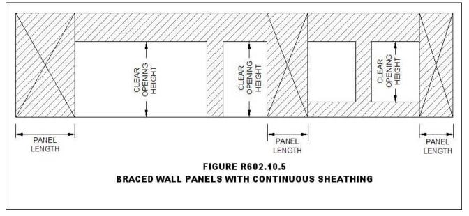
R602.10.5.2 Partial credit. For Methods DWB, WSP, SFB, PBS, PCP and HPS panels between 36 inches and 48 inches in length shall be considered a braced wall panel and shall be permitted to partially contribute towards the required length of bracing in Table R602.10.3(1) and R602.10.3(3), and the contributing length shall be determined from Table R602.10.5.2.
