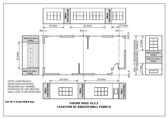
R602.10.2.3 Minimum number of braced wall panels. Braced wall lines with a length of 16 feet (4877 mm) or less shall have a minimum of two braced wall panels of any length or one braced wall panel equal to 48 inches (1219 mm) or more. Braced wall lines greater than 16 feet (4877 mm) shall have a minimum of two braced wall panels.
