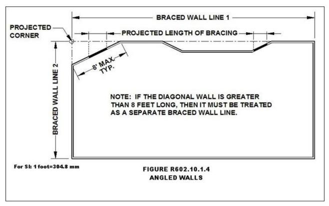
R602.10.2 Braced wall panels. Braced wall panels shall be full-height sections of wall that shall have no vertical or horizontal offsets. Braced wall panels shall be constructed and placed along a braced wall line in accordance with this section and the bracing methods specified in Section R602.10.4.
