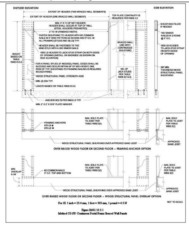
R602.10.3.2 Length of braced wall panels with continuous sheathing. Braced wall panels along a braced wall line with continuous sheathing shall be full-height with a length based on the adjacent clear opening height in accordance with Table R602.10.3.2. Where a panel has an opening on either side of differing heights, the taller opening shall govern when
