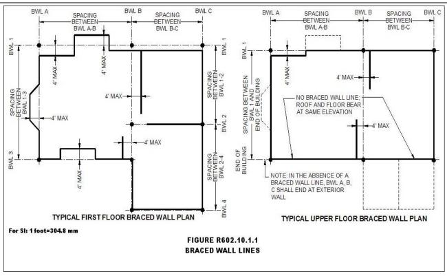
R602.10.1.2 Offsets along a braced wall line. All exterior walls parallel to a braced wall line shall be permitted to offset up to four feet (1219 mm) from the designated braced wall line location as shown Figure R602.10.1.1. Interior walls used as bracing shall be permitted to offset up to four feet (1219 mm) from a braced wall line through the interior of the building as shown in Figure R602.10.1.1.
