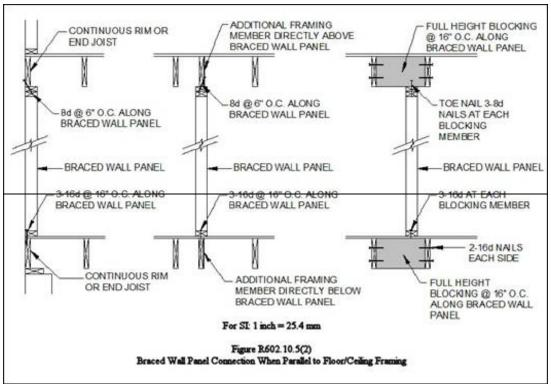
R602.10.6 Braced wall panel support. Braced wall panels shall be supported as follows:
