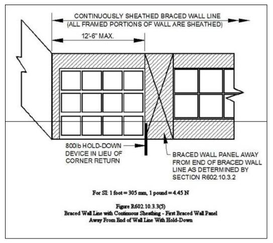
R602.10.4 Braced wall panel finish material. Braced wall panels shall have 1/2 inch thick gypsum board installed on the side of the wall opposite the bracing material and fastened in accordance with Table R702.3.5.
