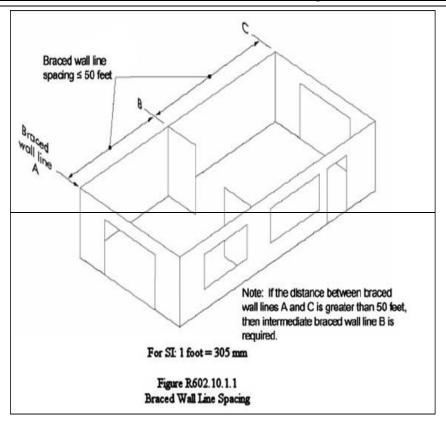
R602.10.1.2 Braced wall panels. Braced wall panels shall be full height sections of wall constructed along a braced wall line to resist lateral loads in accordance with the intermittent bracing methods specified in Section R602.10.2 or the continuous sheathing methods specified in Section R602.10.3. Mixing of bracing methods shall be permitted as follows:
